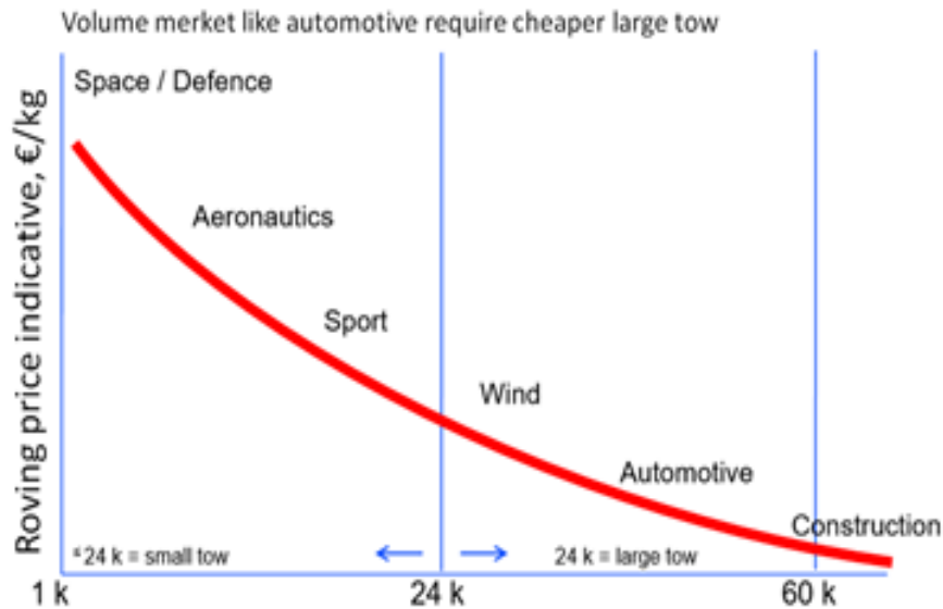
Figure 21. Small tow versus large tow segmentation
